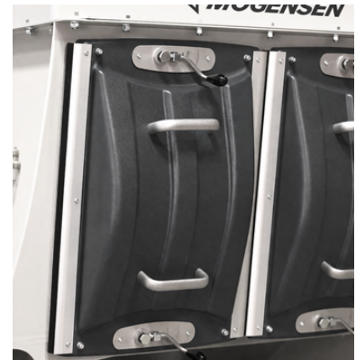
Modularised 0.5 m wide rear covers with 2 quick- release fasteners
