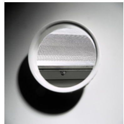
Strategically positioned inspection ports simplify screen cloth change
