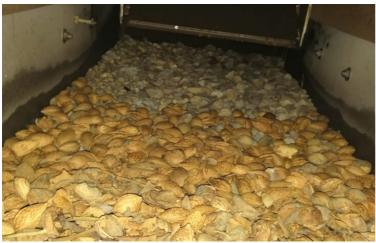
Photo: Interior of the densimetric table (in operation) at the ALLGAIER MOGENSEN test plant.
