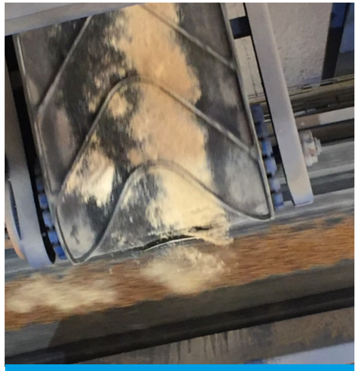
Separated substrate, before discharging the live and dead insects on the belt.
